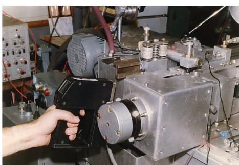
**Fig. 3.** Measurement of temperature in the cutting area
